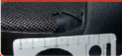
Speaker mesh damage
