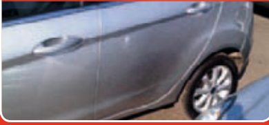
Poor repair: repainted panel does not match
