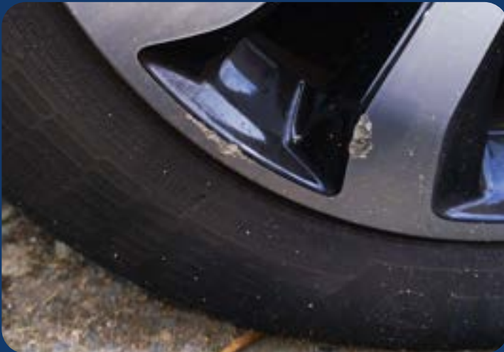
N/S/R alloy spoke face scuffed/corroded
