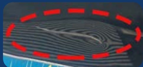
N/S/R door dented/ paint surface broken
