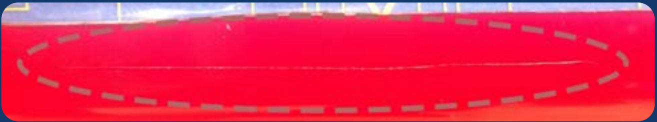
N/S/R door scratched through paint - 25mm >
