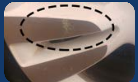
N/S/R alloy spoke face scuffed/corrosion
