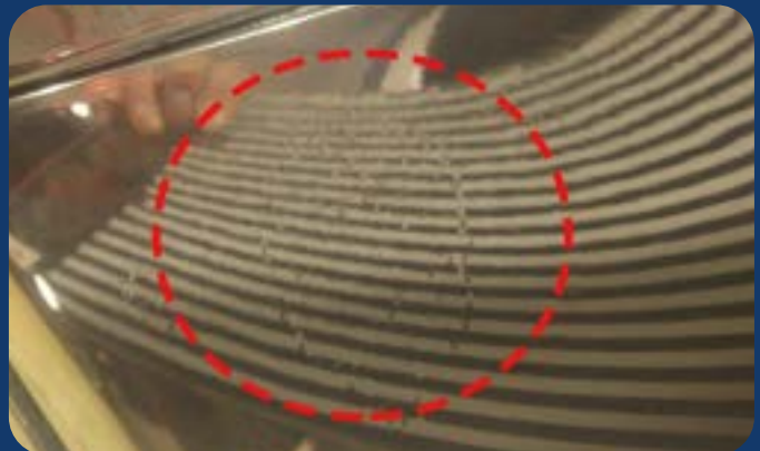
N/S/R bumper - poor paint repair, contamination
