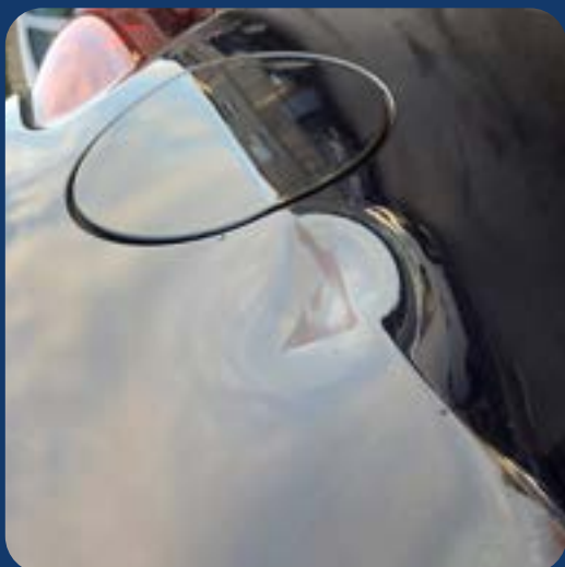
O/S/R door dented through swage line
