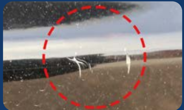
scratches where primer or bare metal is showing
