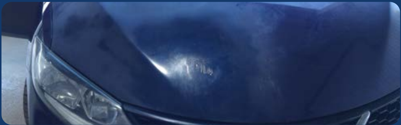
Bonnet - poor paint repair, fillers visible, overspray, runs, etc.
